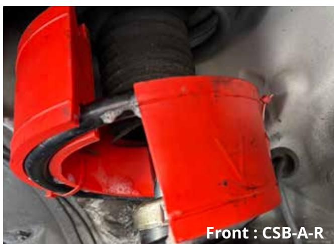
Rear coil spring gap is very narrow, and size E is tight fit. A standard screwdriver will be very helpful to pull the outside ring out of the coil, so the buffer can sit on the coil.
